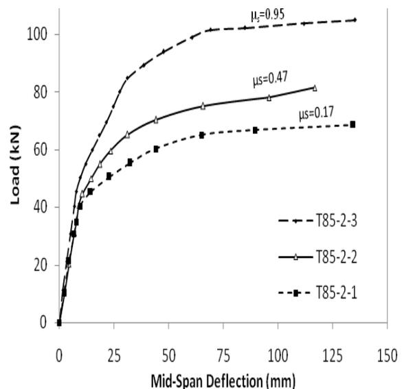
Figure 6-a-Variou non-prestressing steel ratios
