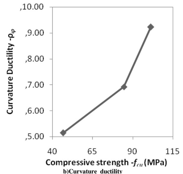
Figure 11- Ductility indices versus concrete compressive strength
