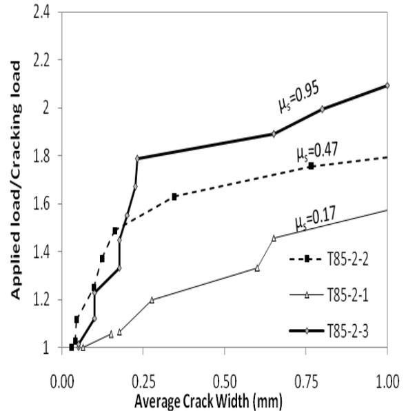
Figure 9- Applied to cracking load ratio vs. crack width for beams with various non-prestressing reinforcement
