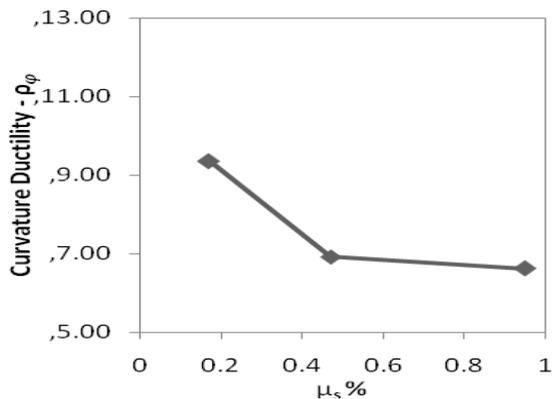
Fig. 12-Curvature ductility index versus non- prestressing reinforcement ratio
