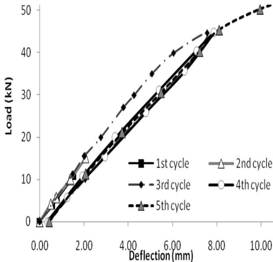
Figure 3 - Typical load-deflection behaviour at mid span deflections during load cycles
