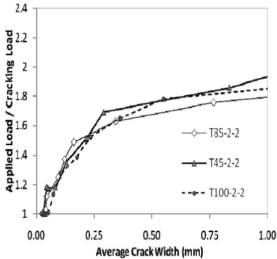
Figure 8- Applied to cracking load ratio vs. crack width for beams with various compressive strengths
