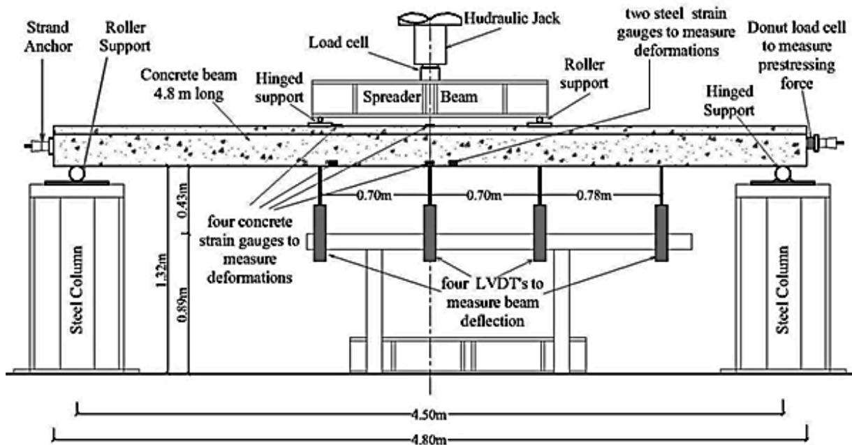
Figure 2- Schematic of the test setup
