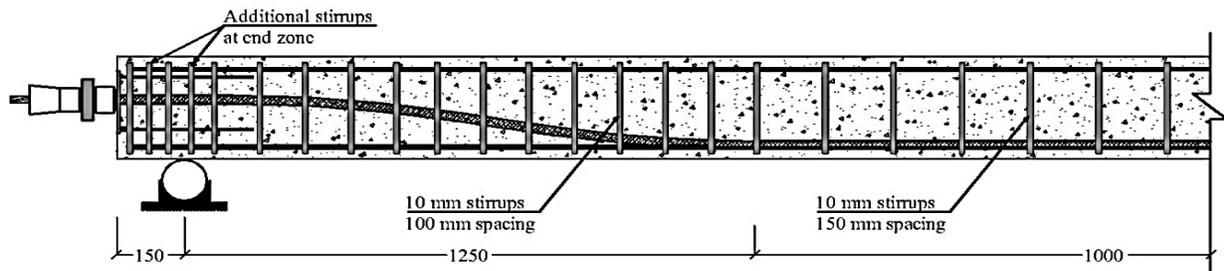
Figure1- Typical sectional elevation for beams
