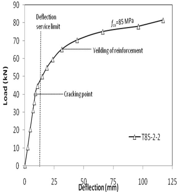
Figure 4 - Load-deflection Behaviour at mid span for control beam
