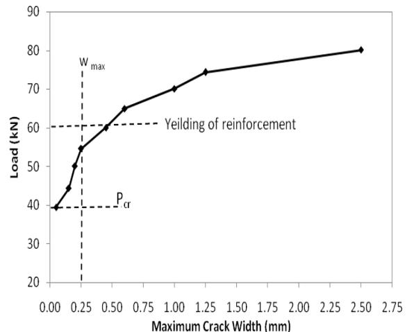
Figure 7- Typical load-crack width relationship for beam T-100-2-2
