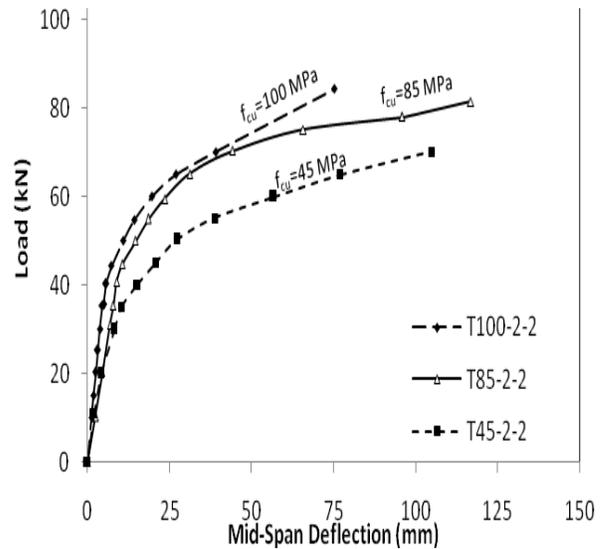
Figure 5- Loa-deflection behaviour at mid span for beams with various compressive strengths
