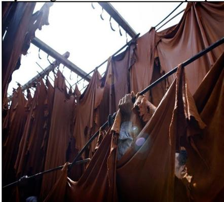
Figure 6 - Air drying of Leather
