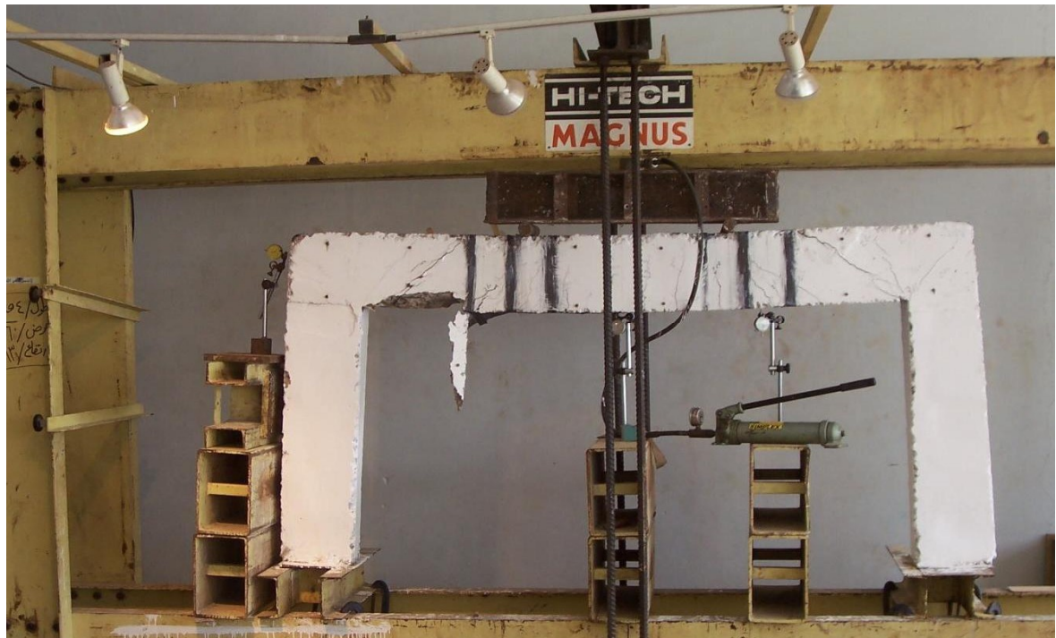
Fig. 6- Failure of Specimen FRP2 due to Concrete Shear Failure Followed by Concrete Cover Separation
