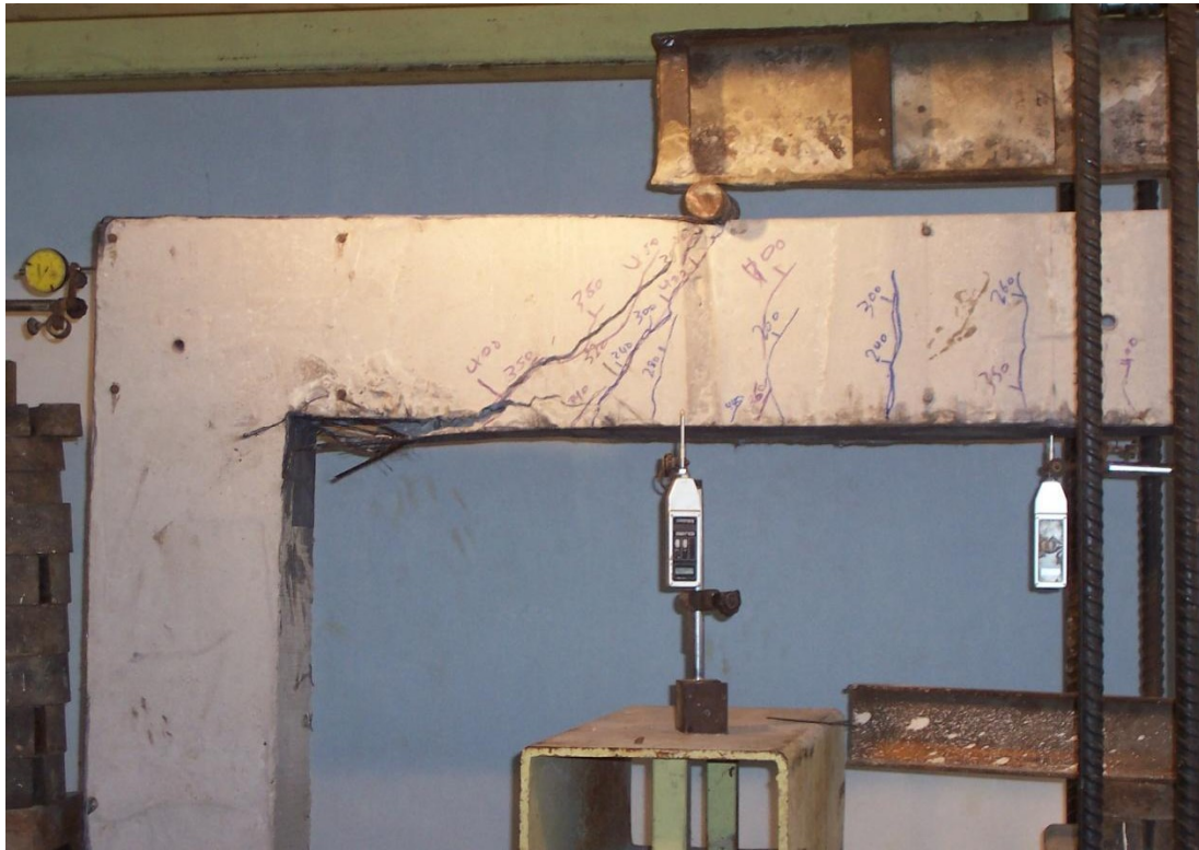
Fig. 5- Failure of Specimen FRP1 due to Concrete Shear Failure
