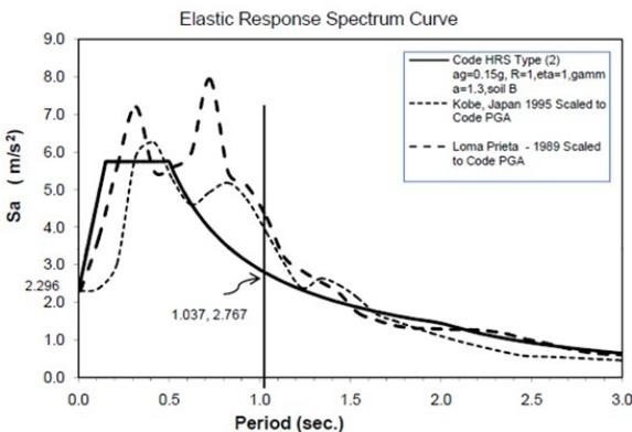
Fig.5- Horizontal Response Spectrum curve of Real Record of Kobe, Japan 1995, Loma Prieta -1999 Scaled to PGA of HRS - Curve as per ECP201 (2008)
