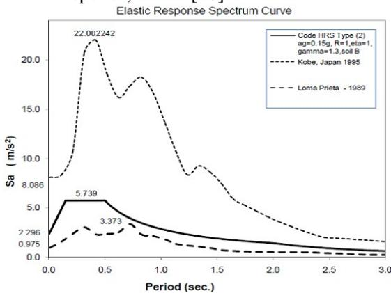
Fig.4-Horizontal Response Spectrum curve of Real Record of Kobe, Japan 1995 , Loma Prieta – 1999 & Code HRS Type (2)
