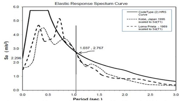
Fig.6- Horizontal Response Spectrum curve of Real Record of Kobe, Japan 1995, Loma Prieta - 1999 Scaled to  $S_a(T_0)$  - as per ECP201 (2008)- of Bridge System(1) ,span-length 25 meters as an example.
