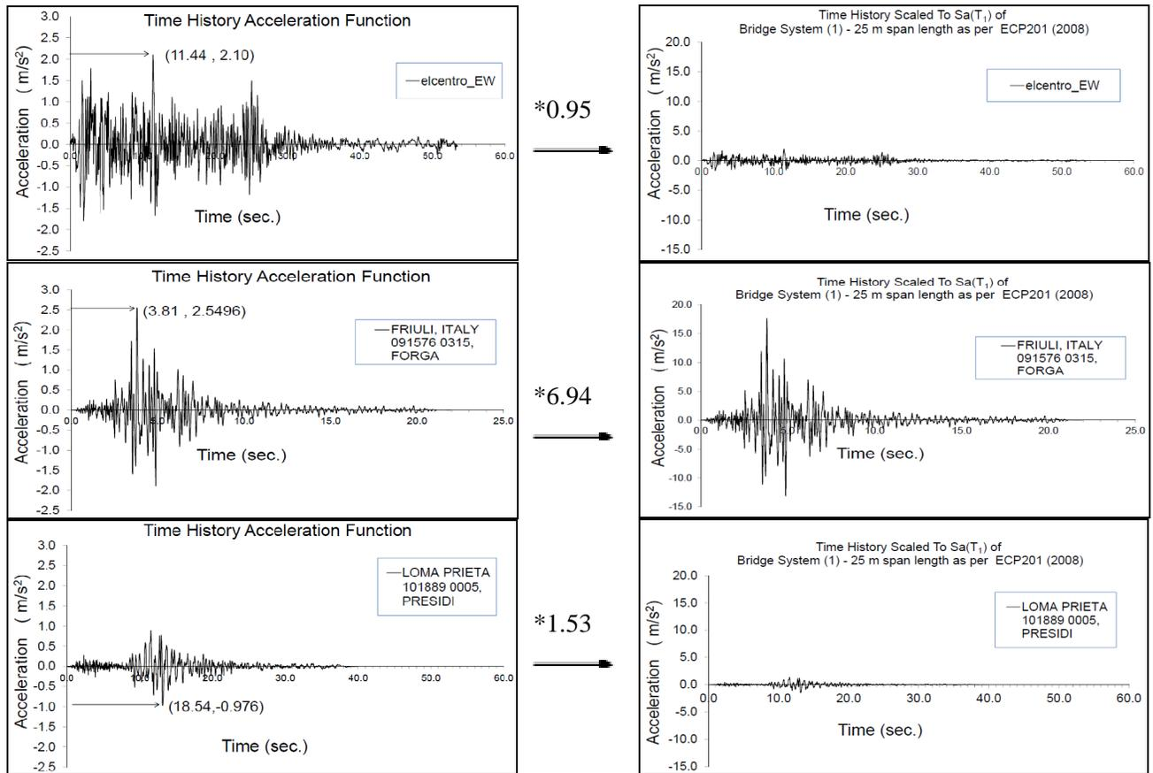
Step (9): Apply these scaled time history functions to Bridge system (1)- 25 meters span-length and get bending moment at section (1) results from time history analysis of each scaled record then take the maximum value (as recommended by ECP201 (2008)).
