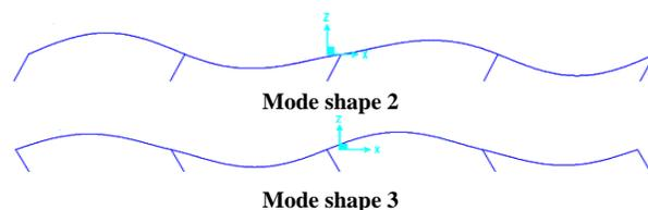
Fig. 3- Mode shape 2&3 of Bridge System (6), 45 meters span-length
