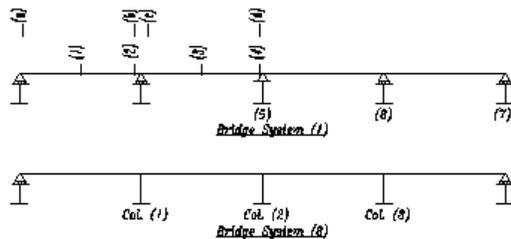
Fig. 2a- The bridge structural systems and critical sections considered in the present study
