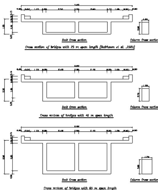
Fig. 2b- Bridges Cross Sections (all shown dimensions are in meters)
