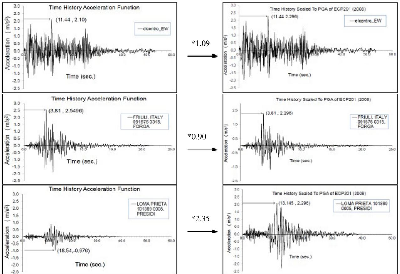
Step (4): Apply these scaled time history functions to Bridge system (1) - 25 meters span-length and get bending moment at section (1) results from time history analysis of each scaled record then
