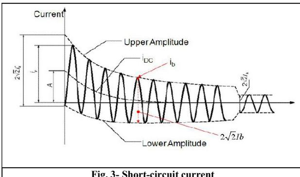
Fig. 3- Short-circuit current
