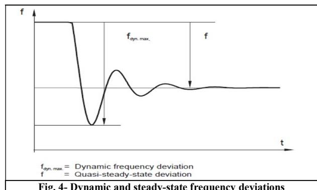
Fig. 4- Dynamic and steady-state frequency deviations
