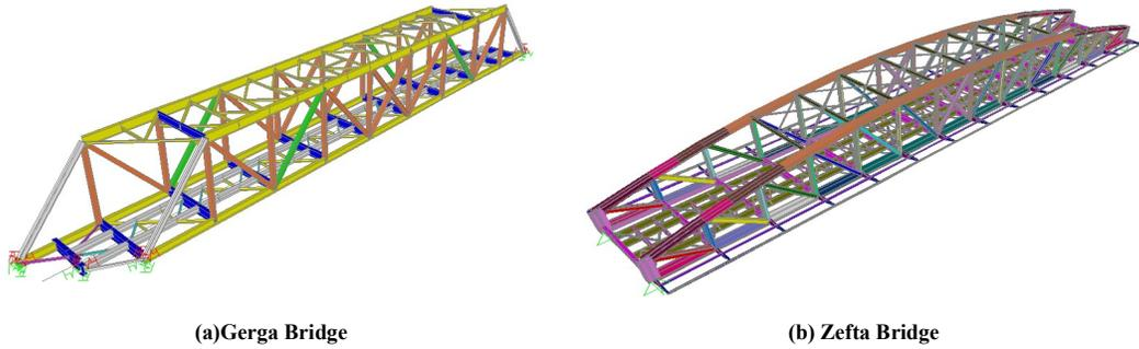
Fig. 4. 3-D finite element model of (a) Gerga & (b) Zifta Bridge
