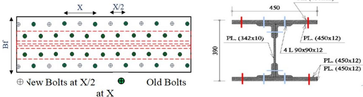
Fig. 9. Tension Buckling Repair
